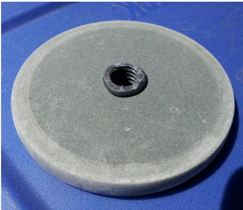
An advantage of tapered threads is that the tighter the wheel gets threaded onto the spindle, the more the lead forms itself into the wheel and on to the tapered thread itself.
