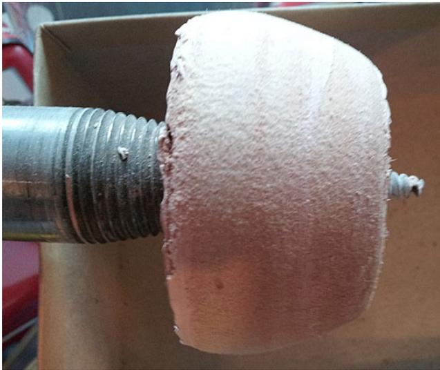
This is the largest tapered threaded spindle I have for my Spatzier lathe. It is approximately 1" at the widest part of the taper.
