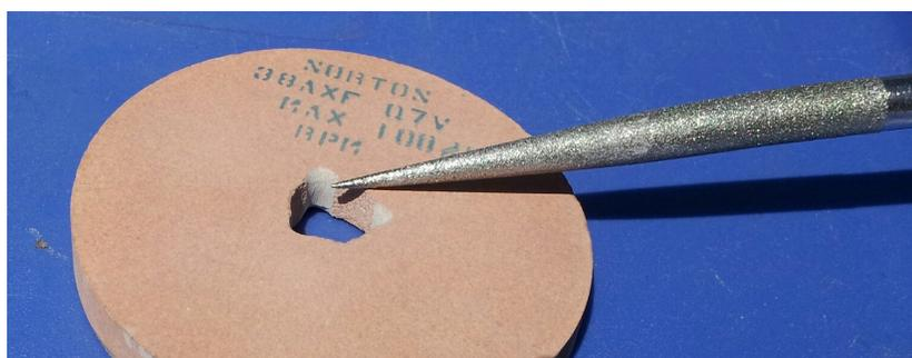
This process may also be done with a tapered round diamond coated file – dry. If the arbor hole is too small for my needs, I redrill it to the desired diameter using a diamond coated core drill on an old drill press. This process is done wet. This roughing up of the arbor hole is necessary for the lead to firmly grip the walls of the arbor hole. It is this firm grip of the
