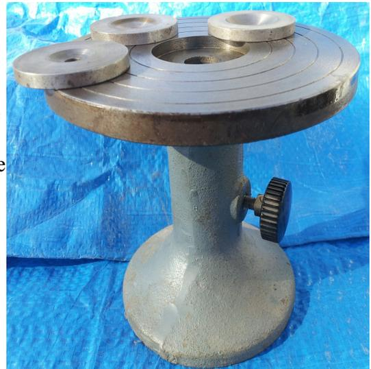
forming this shoulder for better support of larger wheels. I have spindles with several sizes of tapered threads for mounting the small to large wheels.
