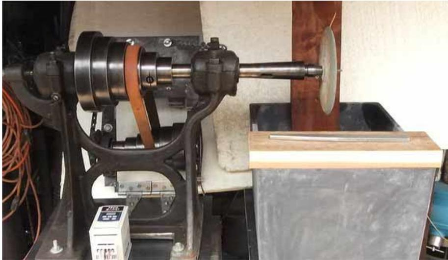
I have setup this lathe with variable speed in addition to the pulley speed changes. This allows for full torque at all speeds. In addition, I have welded up the steel base to hold up to five 8" x 8" x 16" concrete blocks to add mass to the unit. The tub is an old lab sink mounted on a table separate from the lathe.
