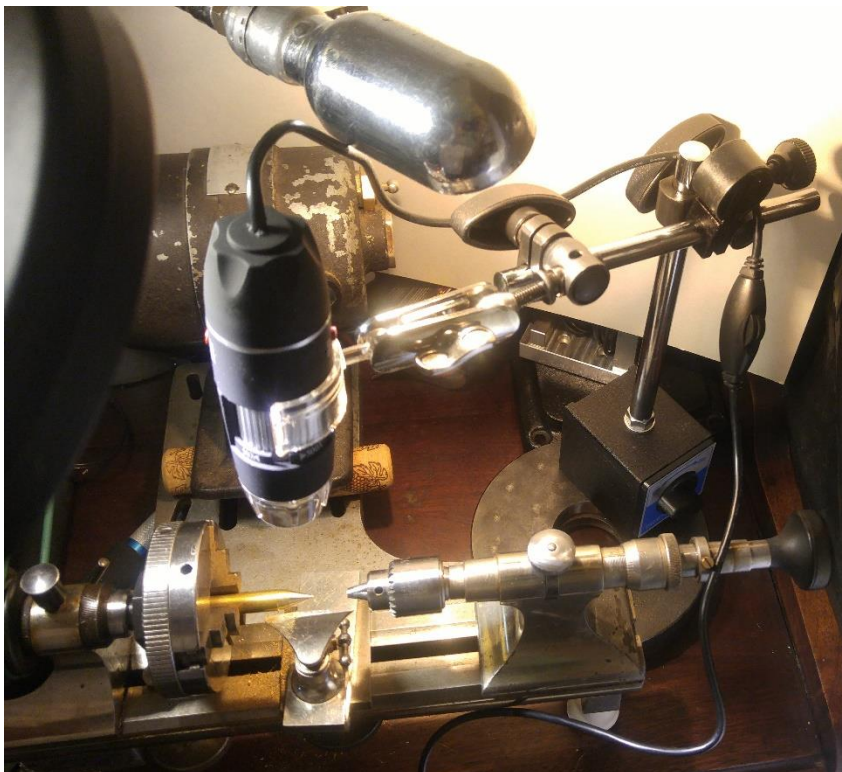
The magnetic mount clamped to the heavy steel ring may clearly be seen.
