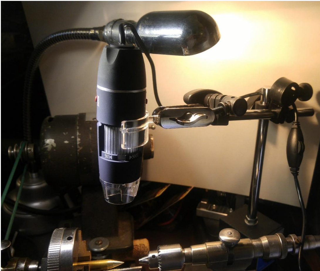
Shown above and below is the microscope suspended above the working area of the WW lathe.
