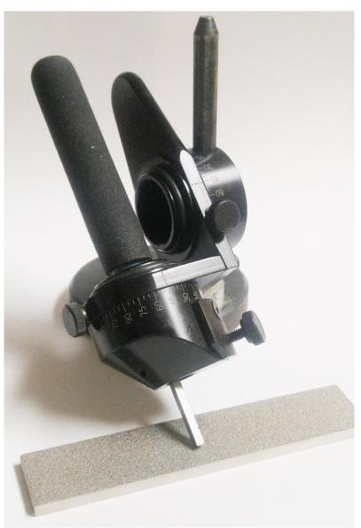
This is the setup for sharpening by hand. The flat diamond bar gets sprayed with Windex and the tool is moved back and forth in an arc.
