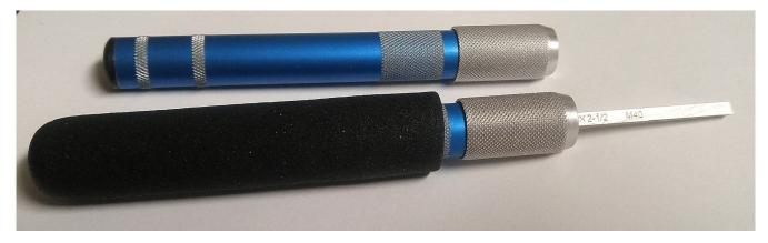
These handles are like super sized pin vises. The tips work like a typical collet. Here is a view of the ends.
