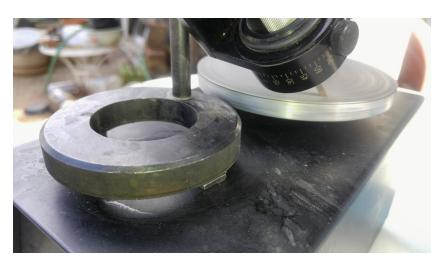
I like to place the fixture ring base on top of several neo magnets to hold it in position. This back and forth grinding is done with each grit until the tip is as needed for lathe work.
