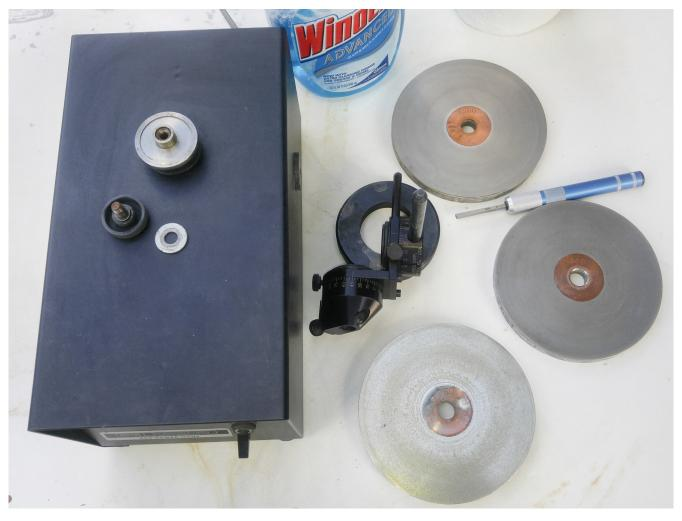
I usually use my old Glendo power hone with an assortment of diamond laps for sharpening. These hones run at a slow speed to prevent any possible overheating. An important part of the equation is the precision tool holder which holds the tooling at the desired angle for grinding.
