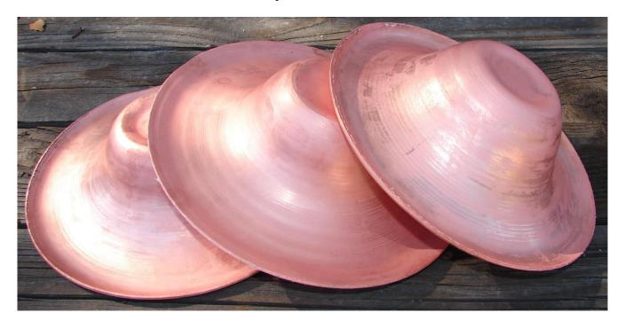
The metal is now spun down to the steel chuck until it again shows signs of work hardening.
