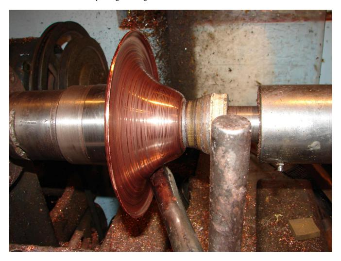
As copper is spun, it work hardens. If spinning of work hardened copper is attempted, the brittle metal will split and the piece will be ruined. Only experience and a developed sense of feel for the metal being worked let the spinner know that it is time to anneal or soften the metal.
