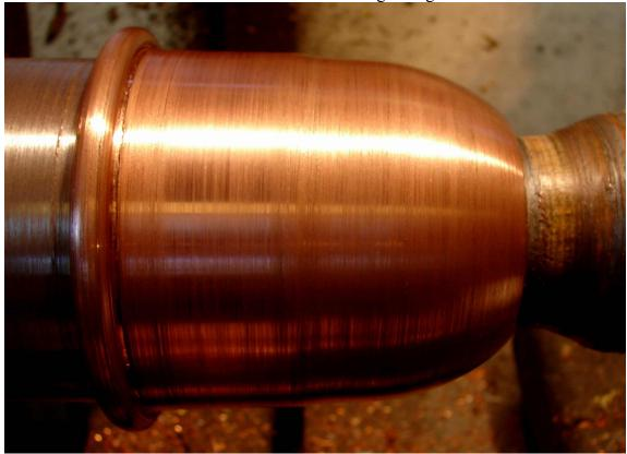
With completion of the mouth bead, the actual spinning was completed.
