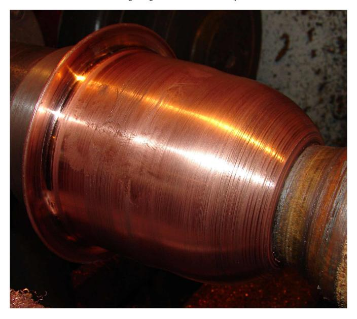
The complete body of the cup was gone over to harden the copper again for durability.
