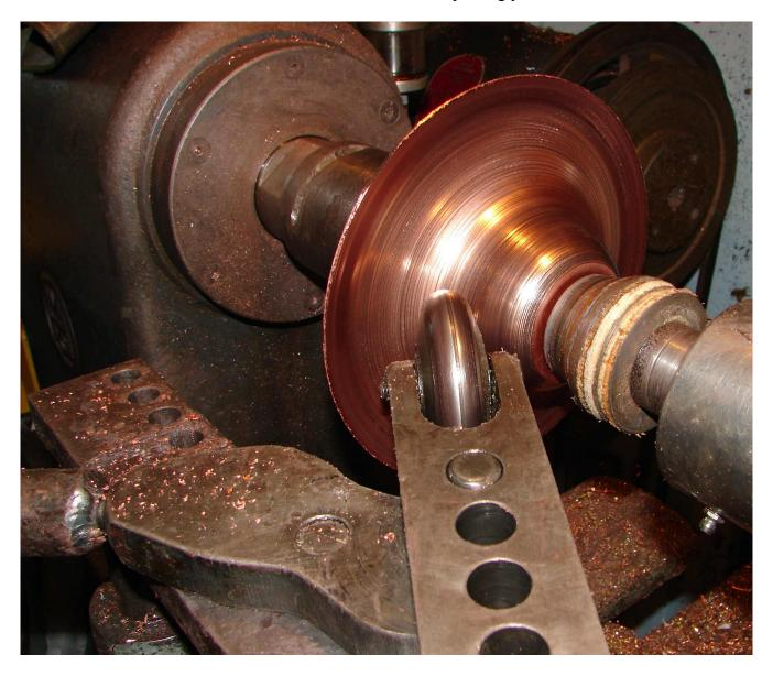
Once the metal is "locked on" to the chuck by being spun tightly to the steel, I switch over to using drag tools for the spinning. Shown below is the tip of a 5' long combination tool smoothing over the roller marks and getting a better fit to the chuck's contour. Drag tools can give a nicer finish and provide a good feel for what the metal is doing. Feel is very important in metal spinning.
