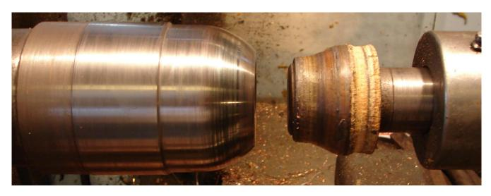
Actually, this thickness of copper is beyond the range of my circle shear. I needed to cut the circles with a large Beverly type of shear. A circle is shown mounted in the lathe. Evidence of the hand shearing may be seen.
