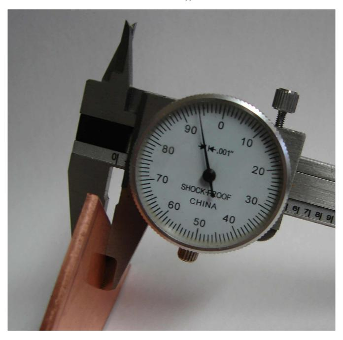
This thickness of copper is very resistant to being spun when compared to the .064" thick copper normally utilized for street cups. This is just shy of being 1/8" thick. This was not to be a simple and easy spinning job.
