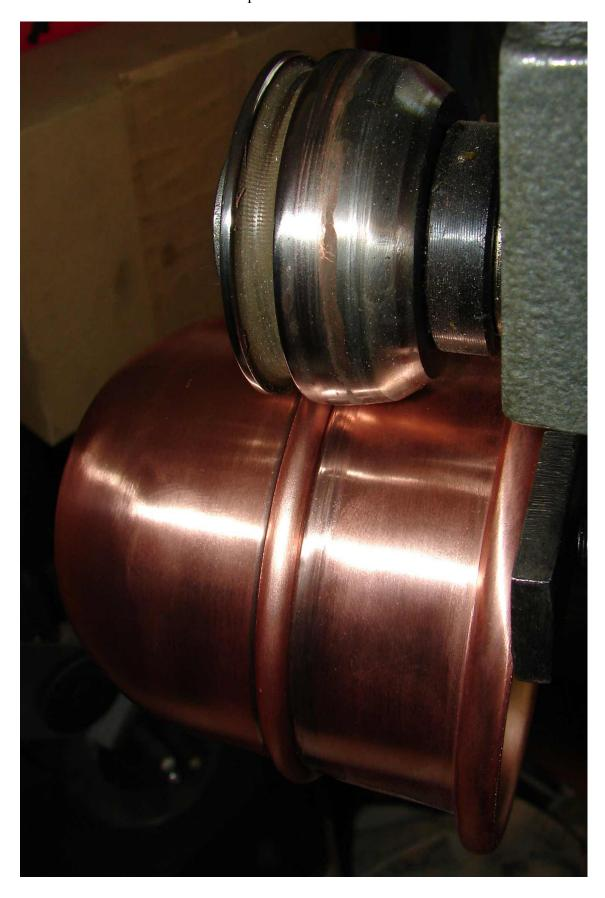
And after the side beads were formed, it was time to see if the cups all stacked correctly. Large cups require some slop in their stack so that a partial vacuum is not created when separating the cups during a performance.
