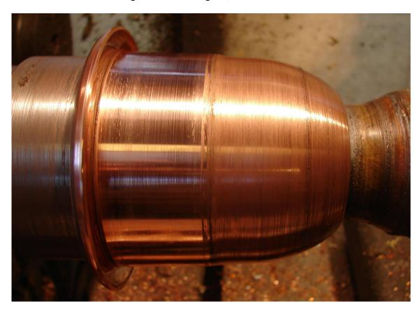
Then the bead is closed to form a good tight bead.
