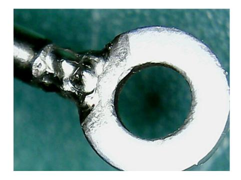
After welding the washers onto the ends of several solenoid shafts, the solenoids can be easily attached to the items that they are to activate. Of course, now I may need to weld small mounting brackets onto the frame of the solenoids for easier mounting.
