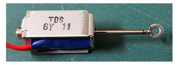
A close up image of the weld illustrates why I worked the metal a bit. The washer and the shaft were both plated and I wanted to be certain that I was welding the base metal.
