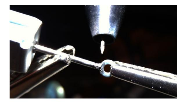
This is the end product right after the welding. The black will be removed with a fine glass fiber brush.
