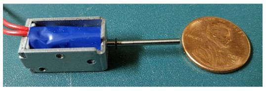
To attach the solenoid to the object that it was to control I chose to micro weld one of these small washers onto the shaft end. Once the washer was attached, I would be able to connect a variety of items to the ends of several solenoids.
